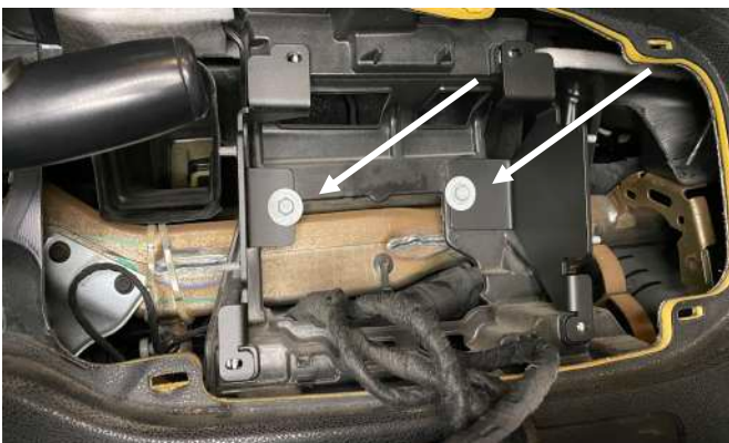
Temporarily remove two (2) OEM screws and attach support bracket with OEM screw as shown. 10mm socket.
