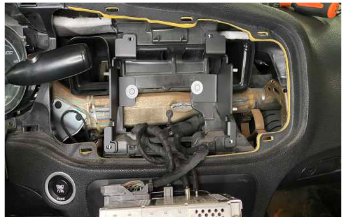
Repeat process for both sides. Make sure brackets fit around radio snug.
