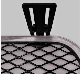
3. Install the Universal Partition Mount L Bracket **(EXPED-LOFT-4)** to the loft and the rear cargo partition.
