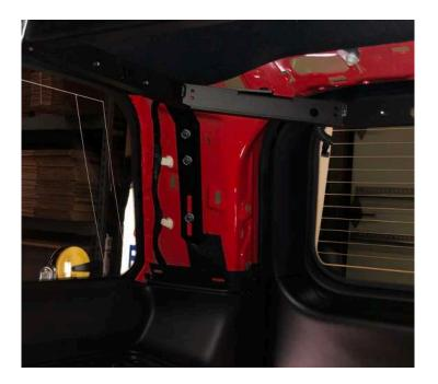
Remove upper rear D-Pillar trim panel on each side to expose factory 3<sup>rd</sup> row seat belt bolt holes (remove 3<sup>rd</sup> row seatbelts if installed in vehicle). For passenger safety, do not use 3<sup>rd</sup> row seating with LOFT installed.
