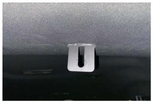
Remove coat hooks on drivers and passenger side and install DS/PS Side crossbar to factory coat hooks. (As shown below) Bolt the 2 Crossbar pieces together using 5/16" hardware. Attach LOFT-3 bracket to cross bar and leave loose until end.
