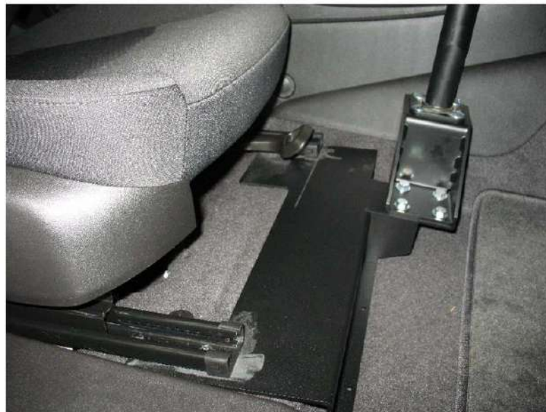
FIG 4 - Offset riser installed on base
