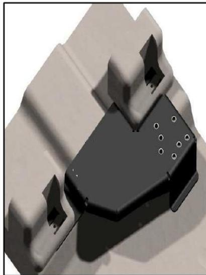
Secure the base under the passenger side seat.
