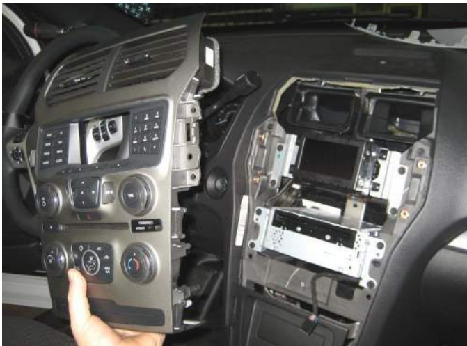
Unplug and remove center control panel
