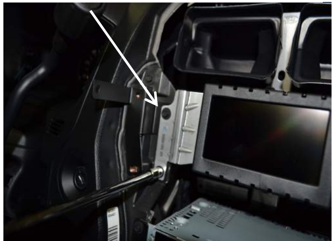
Attach driver and passenger side upper support bracket with OEM display screws. Driver side shown. Torque to 3 Nm (27 in-lbs)
