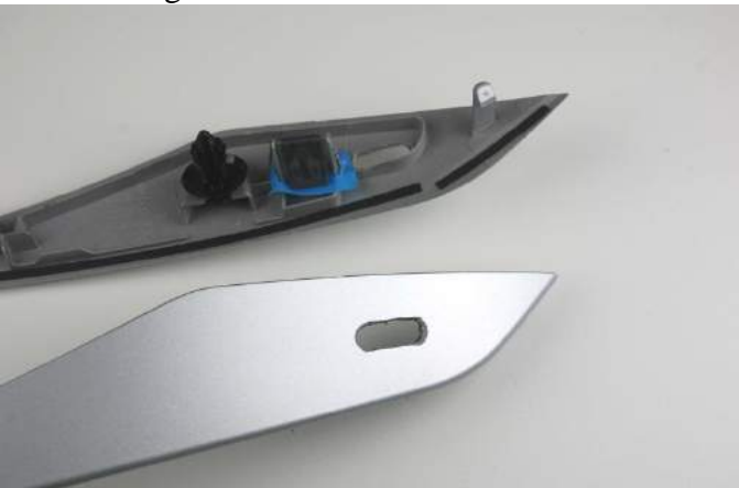
View of upper trim bezels with slot.
