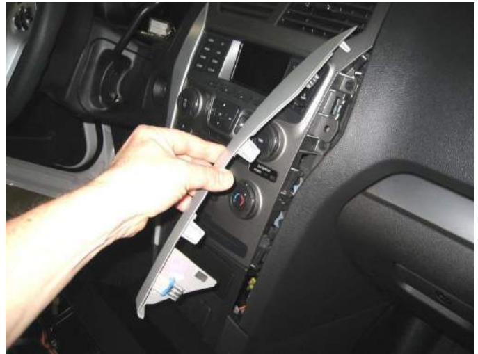
Carefully remove (unsnap) passenger side Dash trim bezel. Trim removal tool and 90° picking tool recommended.
