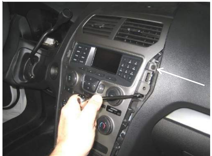
Remove screws holding center control panel. (7mm socket)
