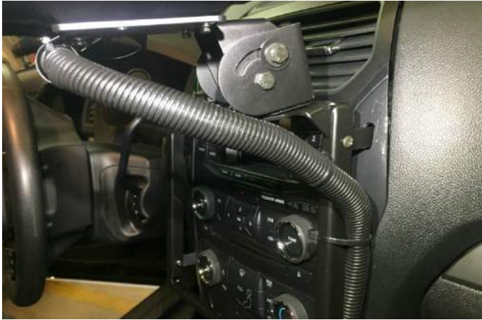
Attach main frame to support brackets with four (4) # 10 x 1/2" Phillips machine screws and star washers. Tighten Hardware.
