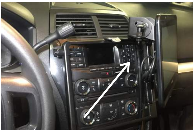
Attach monitor mount adaptors to back of monitor. Attach monitor adaptor to swing door with 1/4" serrated nuts and position as desired. Tighten hardware.
