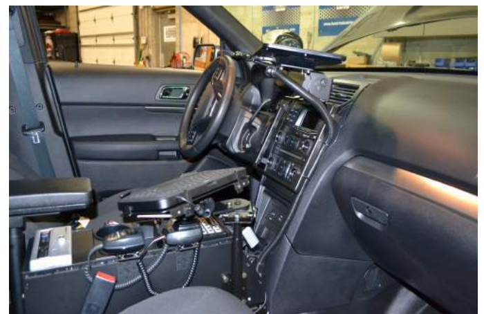
Note: Monitor can be slightly rotated clockwise. Loosen monitor bracket and swivel bracket hardware, turn clockwise and tighten.
