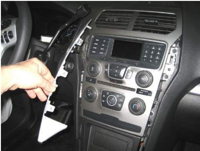
Carefully remove (unsnap) driver side Dash trim bezel.
