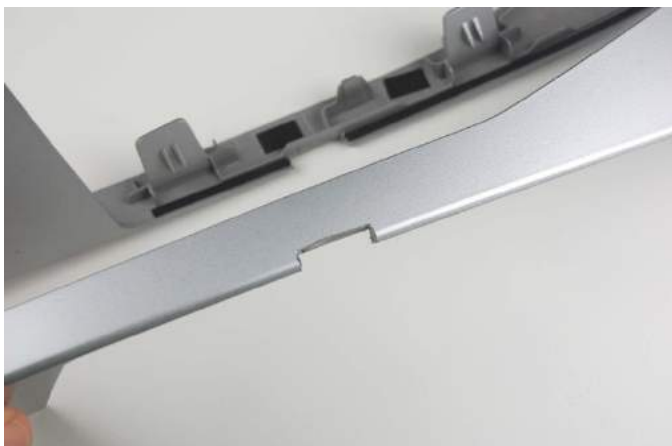
View of trim bezels with notch.
