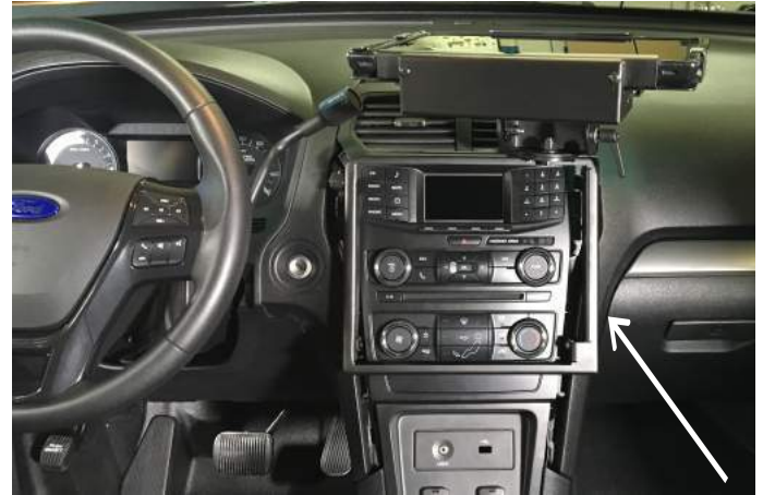
Main assembly is now in place.
