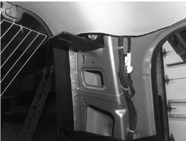
1. Remove upper rear D-Pillar trim panel on each side to expose factory 3<sup>rd</sup> row seat belt bolt holes (remove 3<sup>rd</sup> row seatbelts if installed in vehicle).
