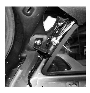
Remove upper rear D-Pillar trim panel on each side to expose factory 3<sup>rd</sup> row seat belt bolt holes. Use supplied Self Threading Bolts and washer to mount L-Bracket (FPIU-LOFT-FB-1) as shown in picture.
