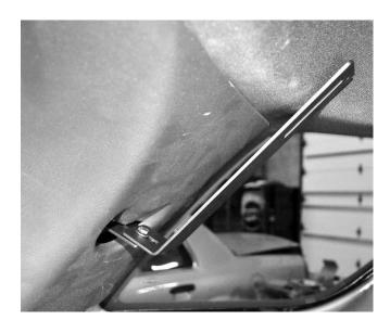
Reattach each trim panel. Loosely install Frame Mount Bracket (FPIU-LOFT-FB-4)
