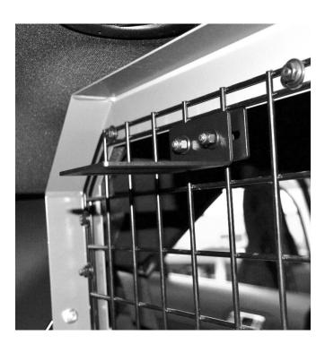
Level the LOFT left to right and front to back. Be sure it is as close to the roof as possible and still fits installed Gun and or equipment.
