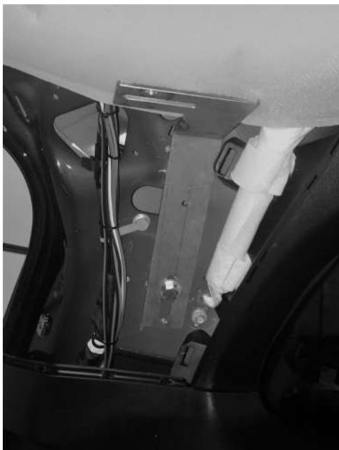
1. Remove upper rear D-Pillar trim panel on each side to expose factory 3<sup>rd</sup> row seat belt bolt holes (remove 3<sup>rd</sup> row seatbelts if installed in vehicle). **For passenger safety, do not use 3<sup>rd</sup> row seating with LOFT installed.**
