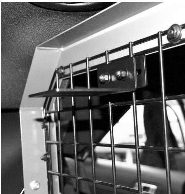
3. Install the Universal Partition Mount L Bracket (**DUR-LOFT-4**) to the loft and the rear cargo partition.
